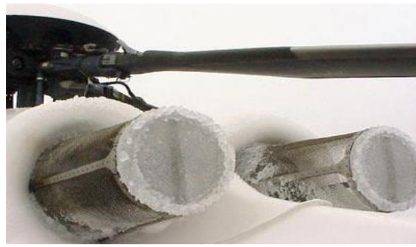
Figure 1. Helicopter air intake protection grids of the AIRBUS H 225 of the SuperPuma family and their icing. (Airbus Helicopters).
