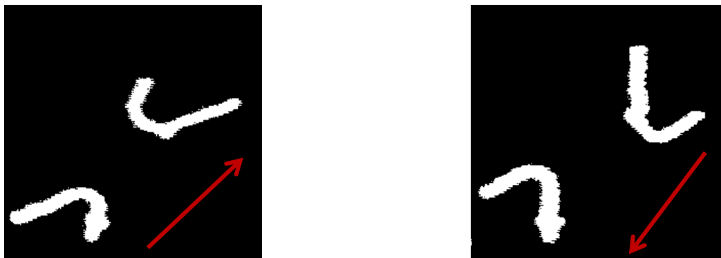
Figure 1. In white the super paramagnetic particle chains, in red the orientation of the external magnetic field. Buckling of two neighbour chains. Distance is \approx 55 \mu\text{m} . Antisymmetric deformation of chains.
