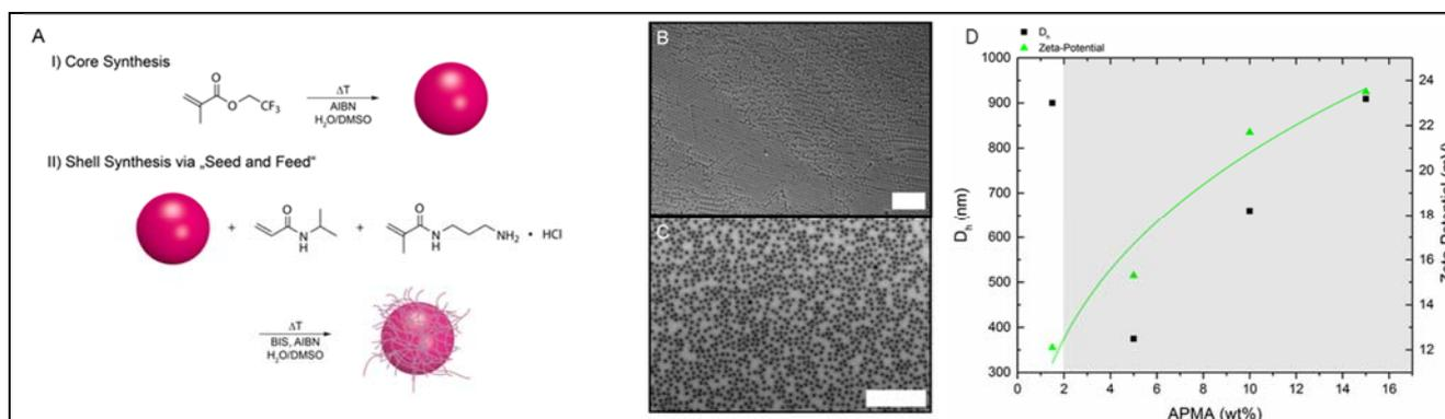
**Figure 1.** a) Synthesis of core and core shell microgels. Electron microscopy images of b) the prepared core and c) core-shell microgels. d) Zeta potential and hydrodynamic radius of the deprotected core-shell microgels in relation to the *N*-(3-aminopropyl)methacrylamide content. Scale bars represent 2  $\mu\text{m}$ .
