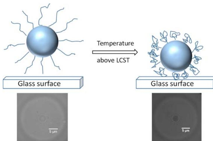
**Figure 1.** Behaviour of thermoresponsive polymers on colloidal probe surface and switchable adhesion to glass surface (left) below lower critical solution temperature (LCST) and (right) above LCST. The microscope images show the increase of the contact area from below (white spot) and above (dark spot) between colloidal probe and glass surface.
